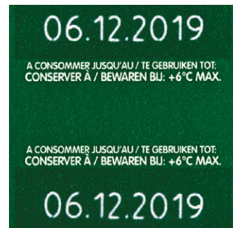
Expiration code Color removal on green foil
